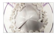
The 1/2 Tablet Cassette is available for certain types of medicine. This special cassette reduces the necessity of manual filling of the trays so that it eventually increases efficiency in the production.
