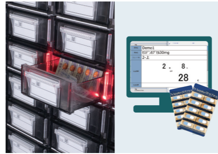
The target case will be unlocked and opened, and the number to be picked will be displayed on the operation screen.
